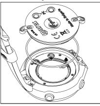
e) Remove the battery by prying it loose with a small flat-head screwdriver.
