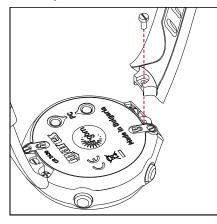
b) Remove the two screws near the padlock symbols. These hold the battery cover in place.
